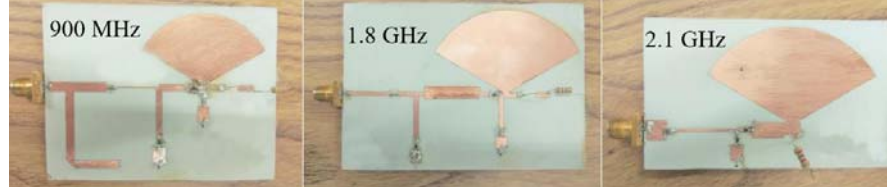
Figure 10. Actual images of three single-band rectifiers.
