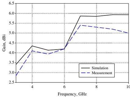
**Figure 12.** Measured and simulated UWB MIMO antenna's gain.
