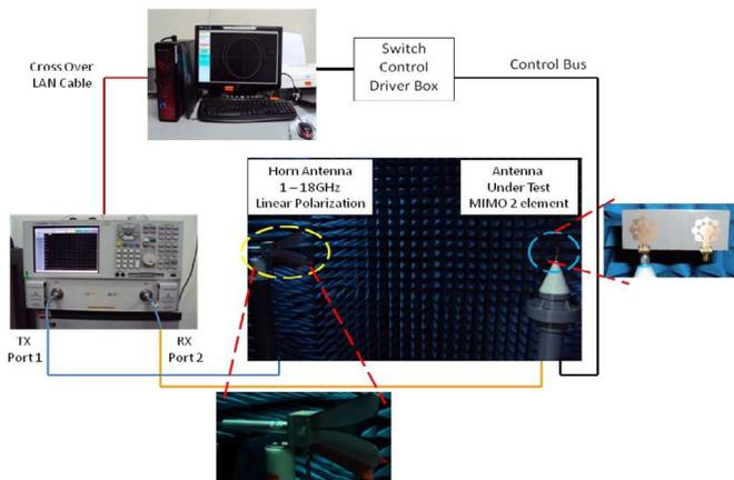
Figure 3. Agilent 2D PNA antenna test system.
