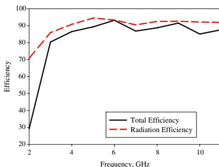
**Figure 9.** Simulated efficiency of the proposed antenna.
