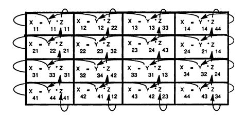
Figure 7.2. Initial assignment of node sections to nodes (and communication pattern).
