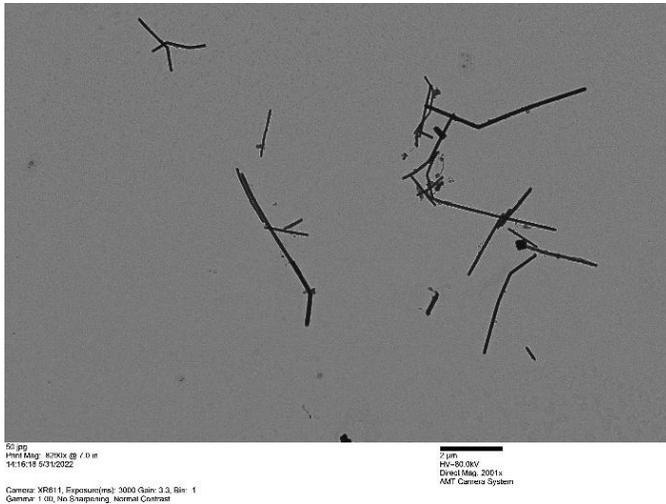
**FIGURE 2.** Sample TEM image of the reduced length measured copper nanofibers.
