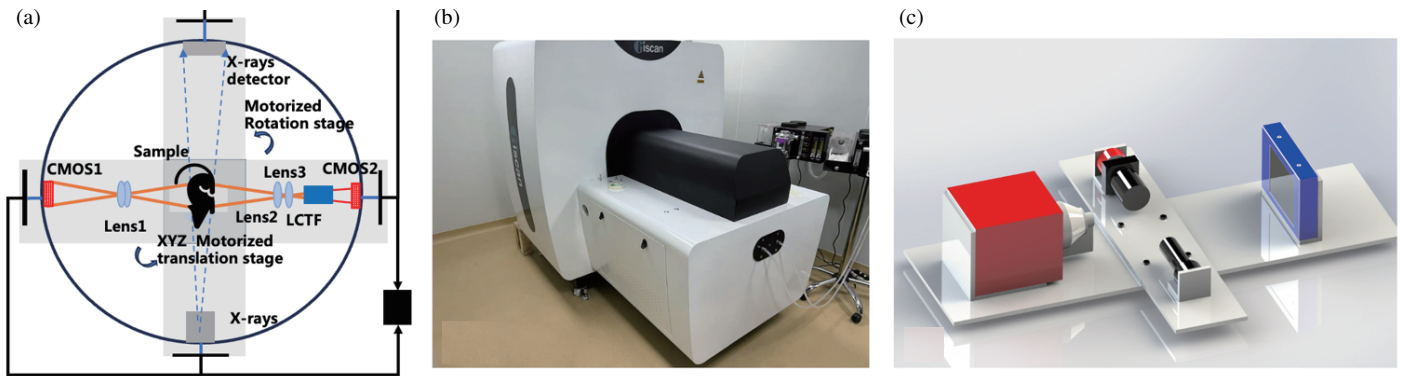
FIGURE 1. (a) Schematic of our dual-modal fluorescence hyperspectral micro-CT system; (b) Physical photograph of the dual-modal system; (c) Internal rotating arm structure.
