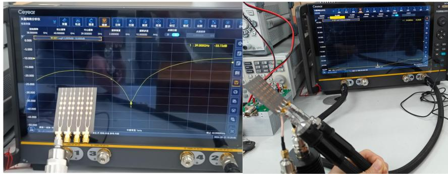
FIGURE 11. Antenna testing diagram.
