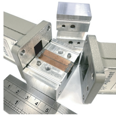
FIGURE 7. The photograph of the back-to-back CPW-to-RWG transition using the integrated resonators and variable housing.
