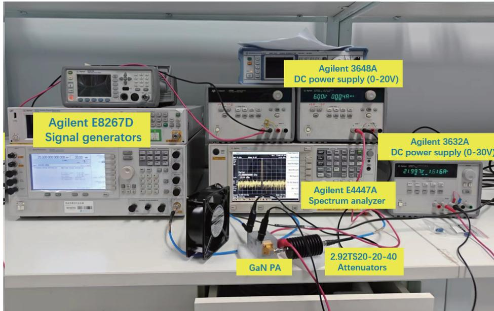
FIGURE 10. Schematic diagram of RF test.
