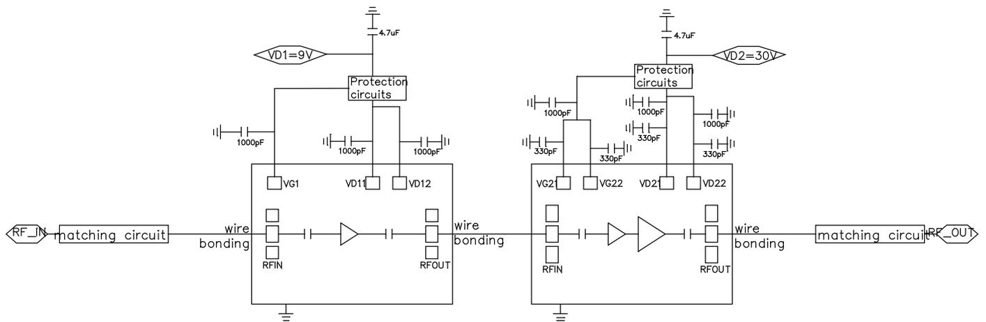
FIGURE 5. Schematic diagram of the protection circuit.
