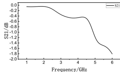
FIGURE 3. RF insertion loss  $S_{21}$  of passive structure of the power amplifier.
