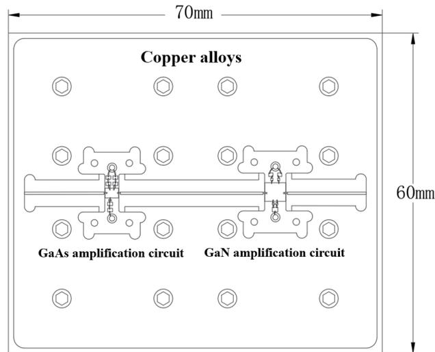
FIGURE 1. The overall assembly layout of the GaN power amplifier.
