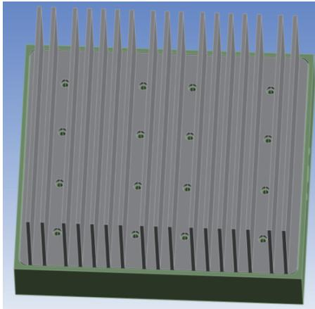
**FIGURE 6.** Fin-shaped heat dissipation structure of the amplifier.
