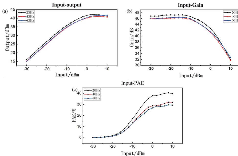
FIGURE 11. (a) Output of PA DUT test. (b) Gain of PA DUT test. (c) PAE of PA DUT test.
