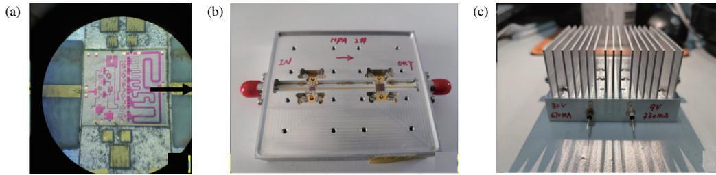
FIGURE 9. (a) GaN die assembly diagram. (b) GaN amplification circuit. (c) GaN power amplifiers.
