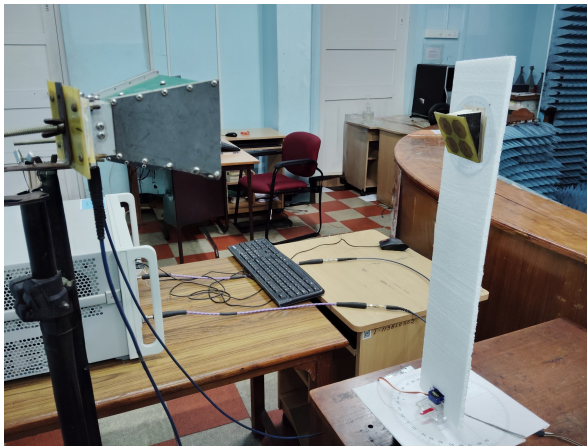
FIGURE 5. Experimental setup in a microwave lab for collecting RFID backscattered signals at varying distances and orientations.
