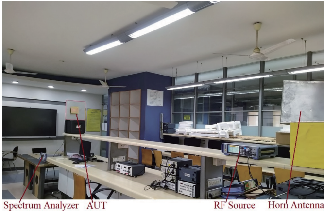
FIGURE 7. Radiation pattern and gain measurement setup.
