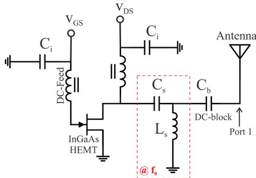
FIGURE 1. Architecture of the proposed self-oscillator antenna.
