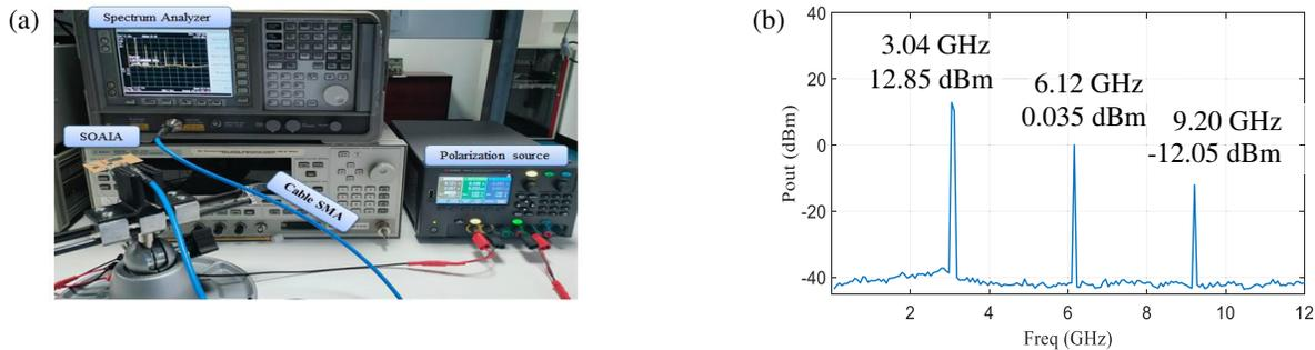
**FIGURE 7.** (a) Measurement setup. (b) Experimental validation of the output power.
