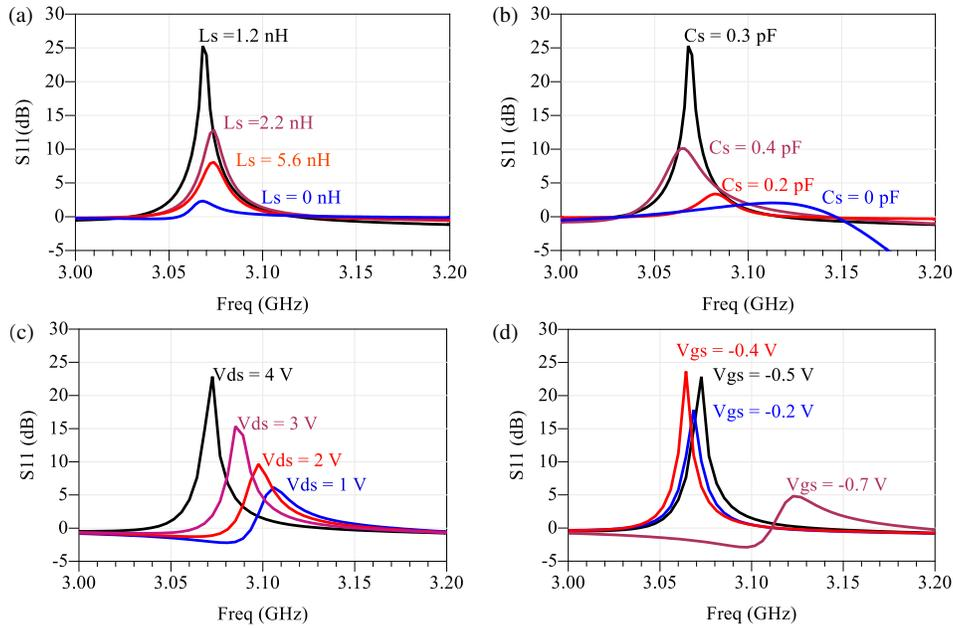
**FIGURE 3.** Analyses of  $s$ -parameters in the self-oscillator antenna proposed (a) and (b) influence of inductance  $L_s$  and  $C_s$  on the reflection coefficient. (c) and (d) influence of polarisation  $V_{ds}$  and  $V_{gs}$  on the reflection coefficient.
