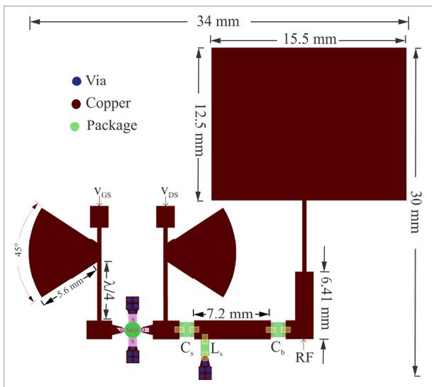
FIGURE 2. Layout of the proposed self-oscillator antenna.
