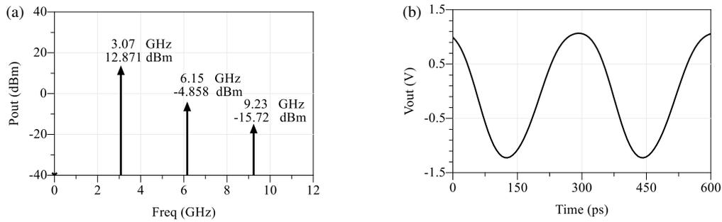
**FIGURE 5.** Harmonic Balance analysis of self-oscillator antenna proposed. (a) Power spectrum of the output as a function of frequency. (b) Output voltage as a function of time domain.
