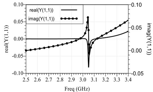
**FIGURE 4.** Verification of the start-up condition for the self-oscillator antenna proposed.
