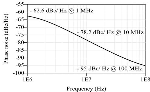
**FIGURE 8.** Phase noise of the self-oscillator antenna proposed.
