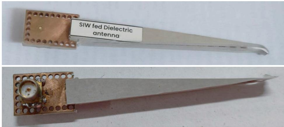
FIGURE 11. Fabricated dielectric rod with tapered grating.
