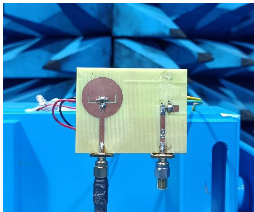
FIGURE 14. Fabricated prototype antenna in an anechoic chamber.
