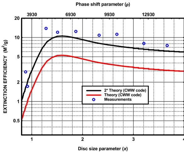
FIGURE 2. Extinction efficiency as a function of size parameter and phase shift parameter for copper discs with thickness of 72 nm for broadside incidence at 35 GHz.
