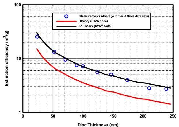
FIGURE 4. Extinction efficiency as a function of thickness for copper discs of size parameter  $x = 1.83$ , for broadside incidence at 35 GHz.
