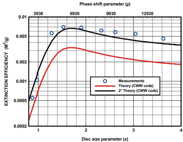
FIGURE 3. Extinction efficiency as a function of size parameter and phase shift parameter for copper discs with thickness of 127 nm for broadside incidence at 35 GHz.
