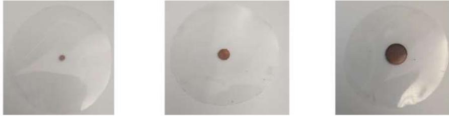
FIGURE 1. Sample pictures of the plated copper discs on mylar diaphragms.
