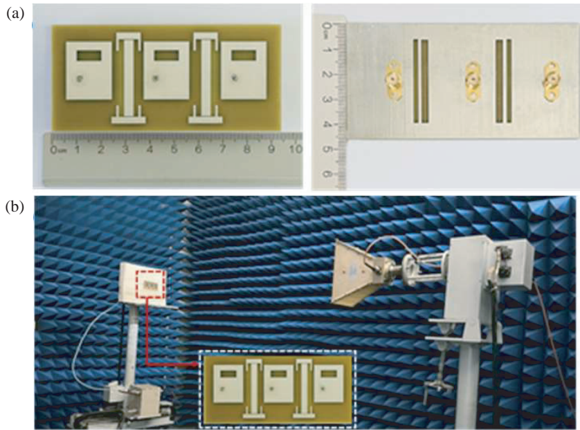
FIGURE 14. (a) Photos of the antenna and (b) the measuring environment.
