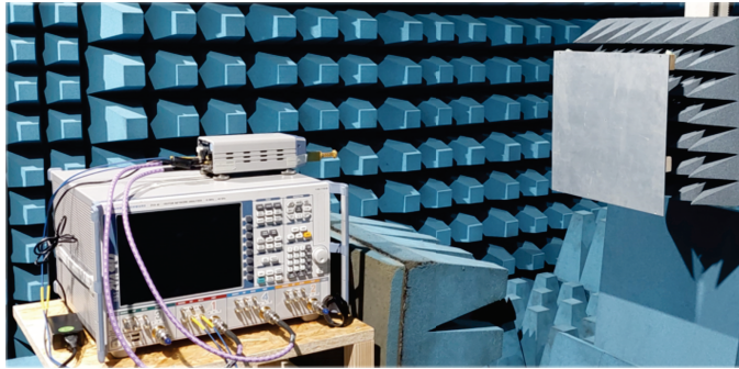
FIGURE 11. Utilized measurement setup in an anechoic chamber. The antenna is focused on the center of the mirror. The table with the analyzer can be rotated.
