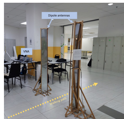
FIGURE 2. Experimental system configuration including vector network analyser (VNA).
