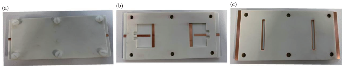
FIGURE 5. The prototype of connection of MSs. (a) Complete assembled interconnection of MSs. (b) Top view without top cover to show the fluidic channel. (c) Bottom view without bottom cover.
