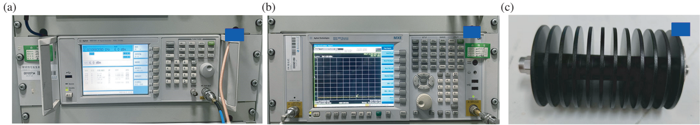
FIGURE 2. (a) N9310A RF signal generator and (b) Agilent N9038A EMI Rx.
