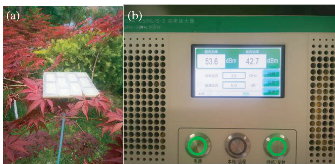
FIGURE 9. Photograph of power capacity measurement and results, (a) the antenna set at the top of tree for power capacity measurement, (b) the monitored forward and reflected power.
