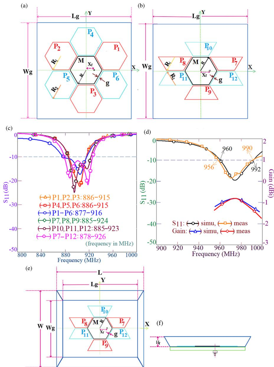
**FIGURE 1.** Gap-coupled configuration of (a) HMSAs and (b) H-HMSAs, and (c) simulated  $S_{11}$  BW plots for gap-coupled combinations of fed and parasitic HMSA and H-HMSAs, (d)  $S_{11}$  BW and gain plots for optimum design of gap-coupled H-HMSAs on finite ground plane, (e) top and (f) side view of gap-coupled H-HMSAs employing cavity-backed structure.
