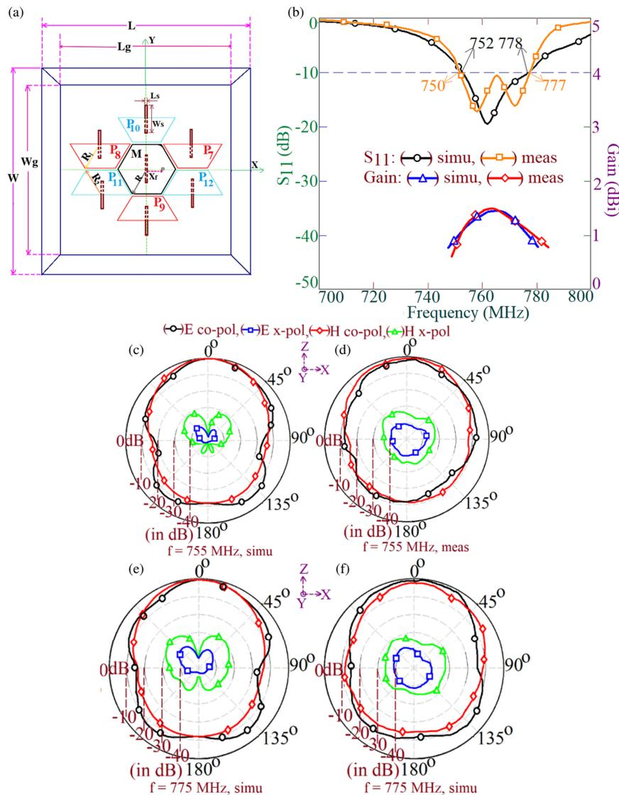
**FIGURE 5.** (a) Gap-coupled H-HMSAs backed by slot cut cavity-backed design, its (b)  $S_{11}$  BW and gain plots and its (c)–(f) radiation pattern nearer to band start and stop frequencies of the BW.
