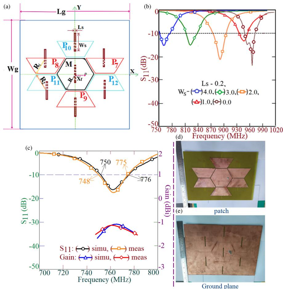
**FIGURE 4.** (a) Gap-coupled H-HMSAs backed by slot cut ground plane, its (b)  $S_{11}$  plots for varying ground plane slot width  $W_s$ , (c)  $S_{11}$  BW and gain plots for optimum design, fabricated prototype showing (d) patch and (e) slot cut ground plane.
