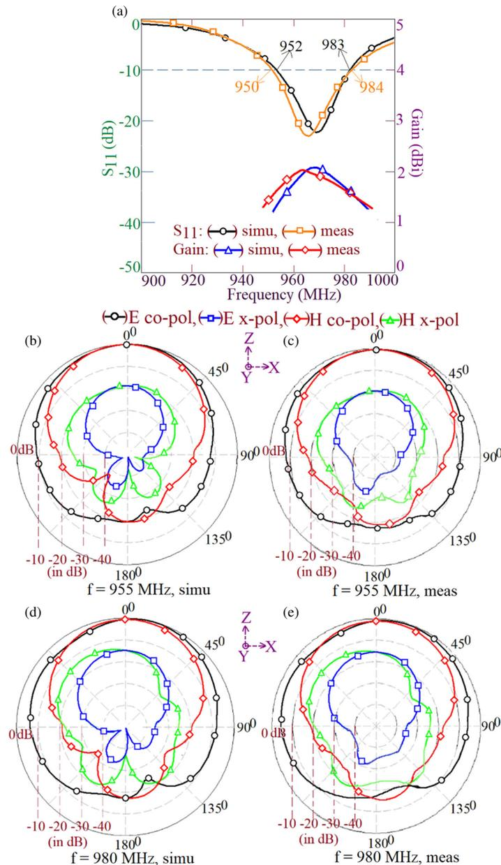
**FIGURE 2.** (a)  $S_{11}$  BW and broadside gain plots and (b)–(e) radiation pattern nearer to band start and stop frequencies of BW for gap-coupled HMSA with H-HMSAs employing cavity-backed structure.
