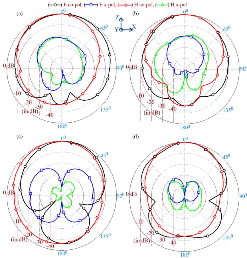
**FIGURE 6.** Simulated radiation pattern plots at the center frequency of  $S_{11}$  BW for gap-coupled configurations of HMSA with H-HMSAs. (a) HMSA gap-coupled with H-HMSAs. (b) Cavity backed HMSA gap-coupled with H-HMSAs. (c) HMSA gap-coupled with H-HMSA backed by slot cut ground plane. (d) Cavity backed HMSA gap-coupled with H-HMSAs backed by slot cut ground plane.
