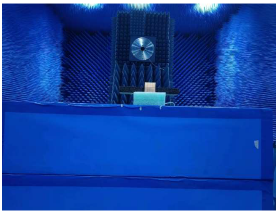
FIGURE 11. Antenna measurement scene.
