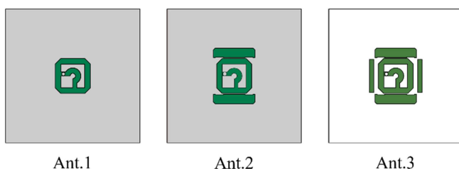
FIGURE 2. Design process of the proposed antenna.
