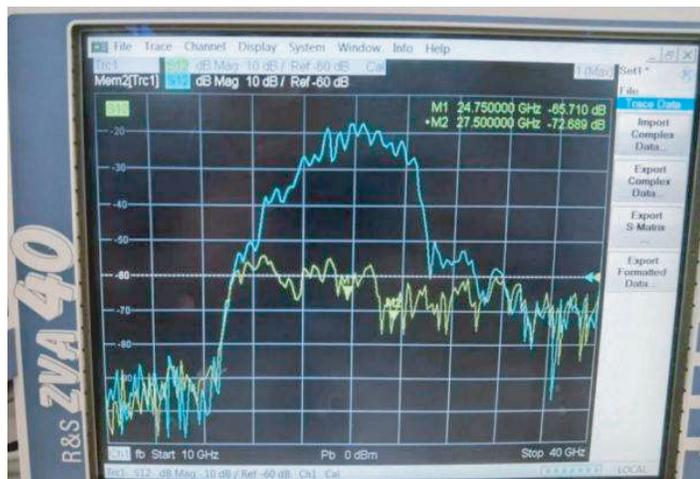
FIGURE 12. Frequency band testing of the active antenna.
