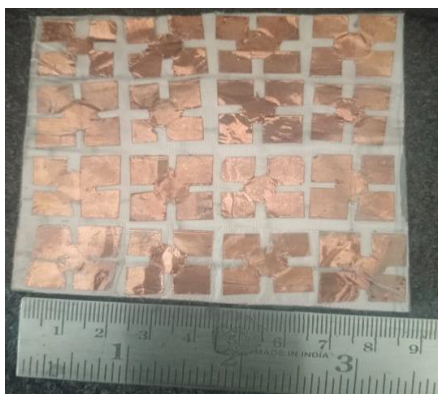
FIGURE 13. Fabricated model of the proposed AMC on Teflon material.
