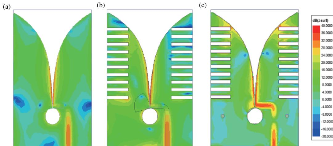
**FIGURE 5.** Current density at 5 GHz. (a) SSVA, (b) corrugated-SSVA, and (c) corrugated-DSVA.
