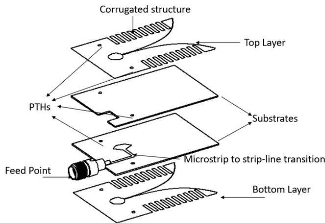
FIGURE 2. Geometry of the proposed antenna.
