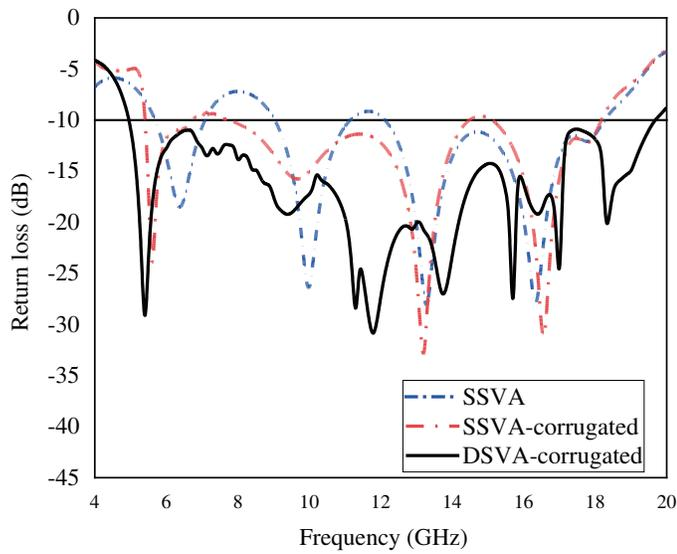
**FIGURE 7.** Comparison in simulated return losses of SSVA, corrugated-SSVA, and corrugated-DSVA.
