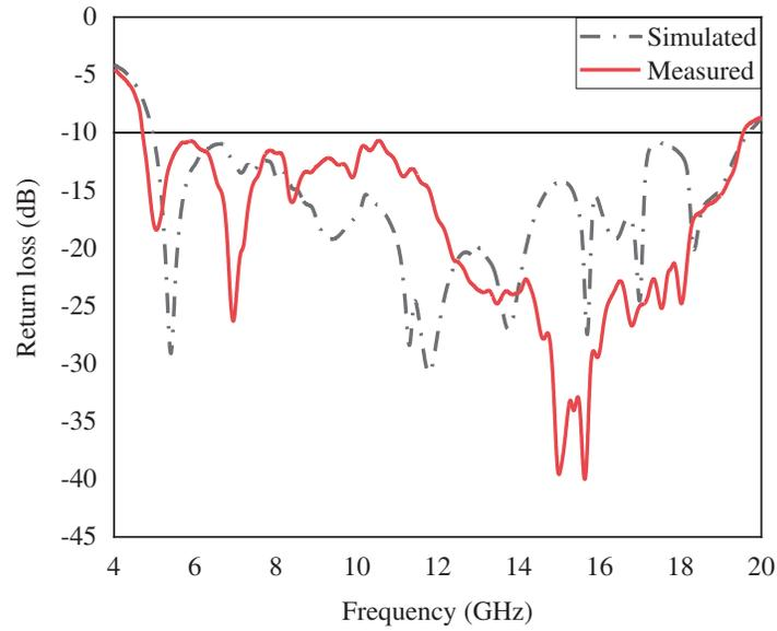
**FIGURE 11.** Simulated and measured return losses (dB) of the proposed antenna.
