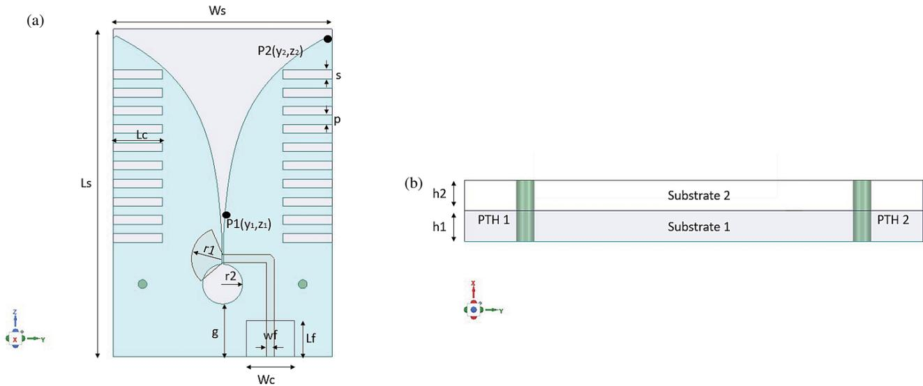
FIGURE 1. Proposed antenna (a) top view, and (b) cross-sectional view.
