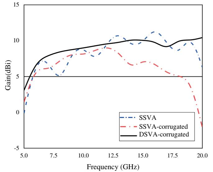
**FIGURE 8.** Comparison in simulated gains (dBi) of SSVA, corrugated-SSVA, and corrugated-DSVA.
