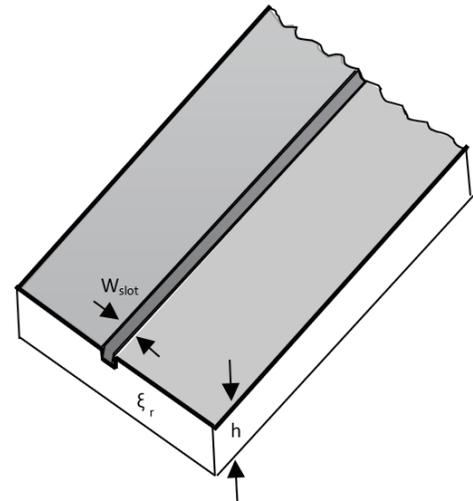
FIGURE 3. Microstrip slot line configuration.
