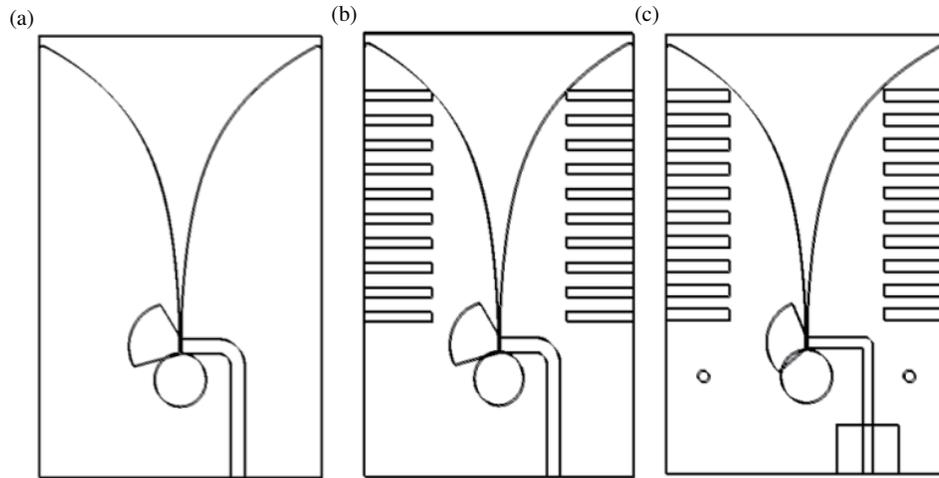
**FIGURE 4.** Antenna configurations. (a) SSVA, (b) corrugated-SSVA, and (c) corrugated-DSVA.
