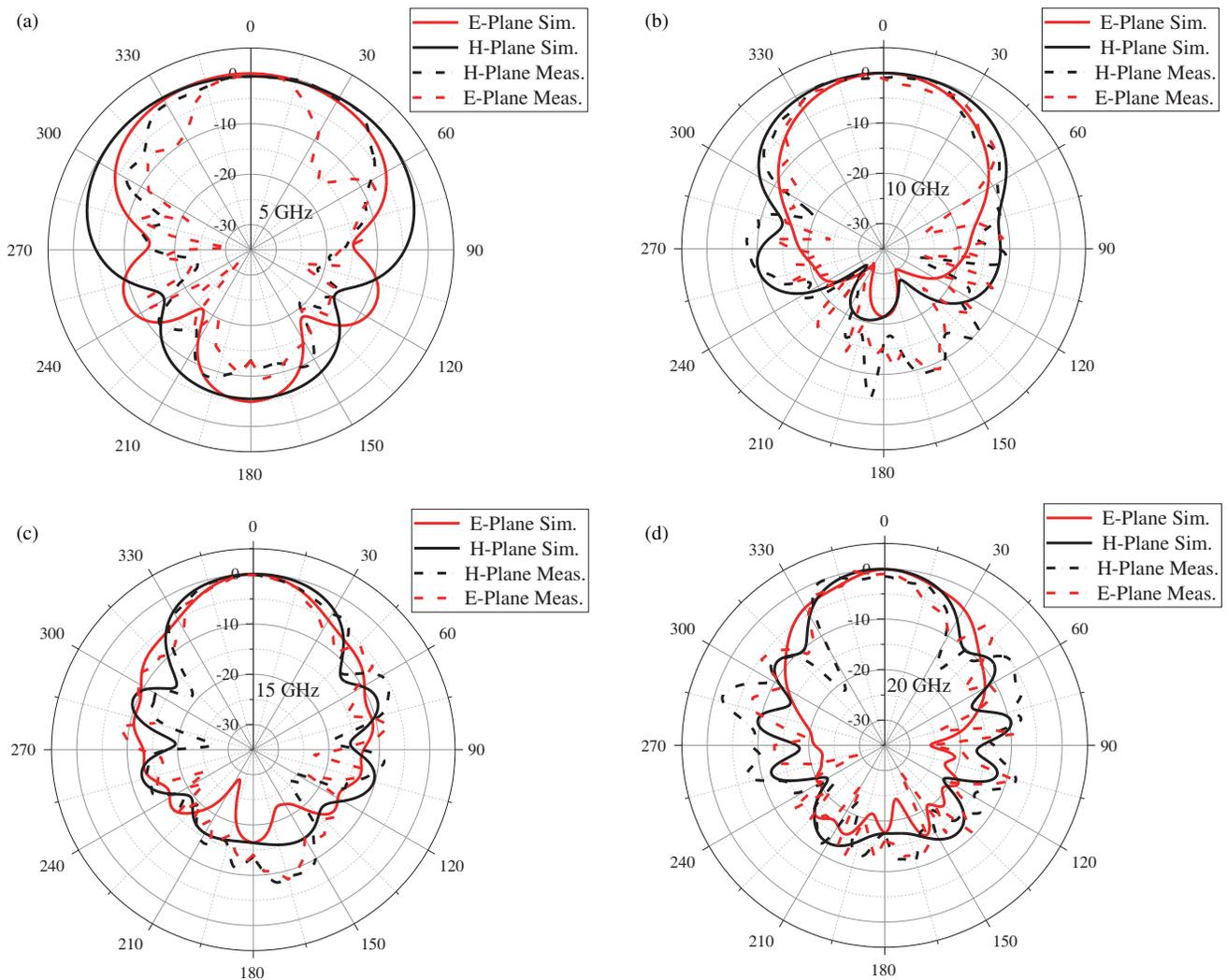
**FIGURE 12.** Simulated and measured radiation patterns of the proposed Antenna. (a) 5 GHz, (b) 10 GHz, (c) 15 GHz, and (d) 20 GHz.
