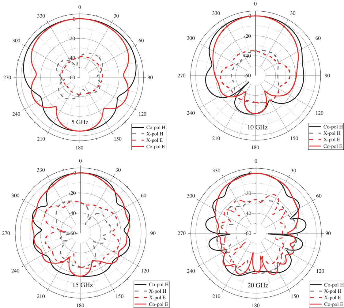
**FIGURE 9.** Simulated radiation pattern of proposed antenna in *E* and *H* plane.
