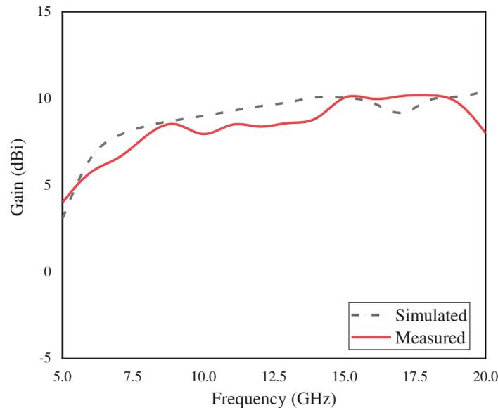
**FIGURE 13.** Simulated and measured gain profiles of the proposed antenna.
