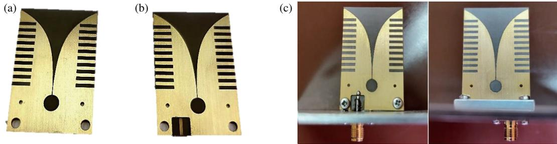
FIGURE 10. Photograph of fabricated PCB and assembled antenna, (a) top Layer, (b) bottom Layer, (c) assemble antenna.
