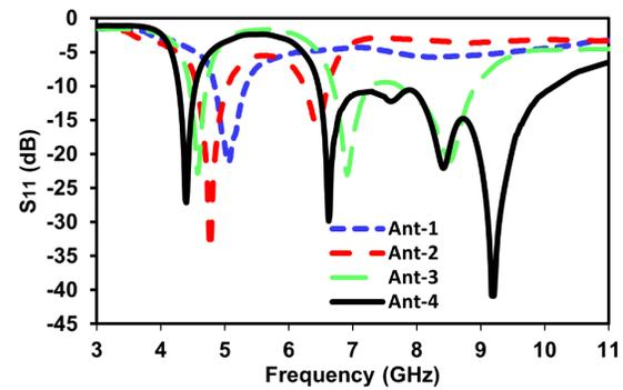
TABLE 2. Step-by-step reflection coefficient improvement of proposed single element antenna.
