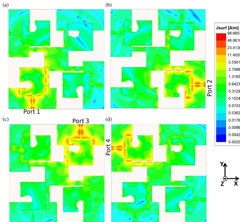
FIGURE 6. Current density of the proposed quad-element MIMO antenna at 4.40 GHz when (a) port-1 excited, (b) port-2 excited, (c) port-3 excited, (d) port-4 excited.
