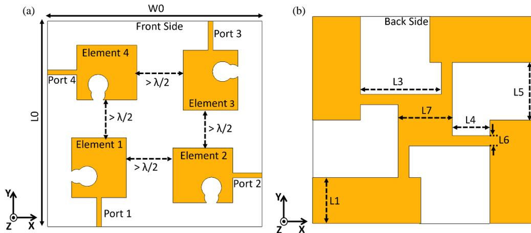
FIGURE 4. Structure of proposed quad-element interconnected ground-based MIMO antenna: (a) front side, (b) back side. Dimensions ( $L0 = W0 = 120$  mm,  $L1 = 26.60$  mm,  $L3 = 44.90$  mm,  $L4 = 20.90$  mm,  $L5 = 33.40$  mm,  $L6 = 6.0$  mm,  $L7 = 30$  mm).
