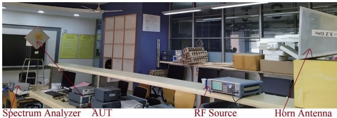
FIGURE 6. Radiation pattern measurement setup with the fabricated antenna.
