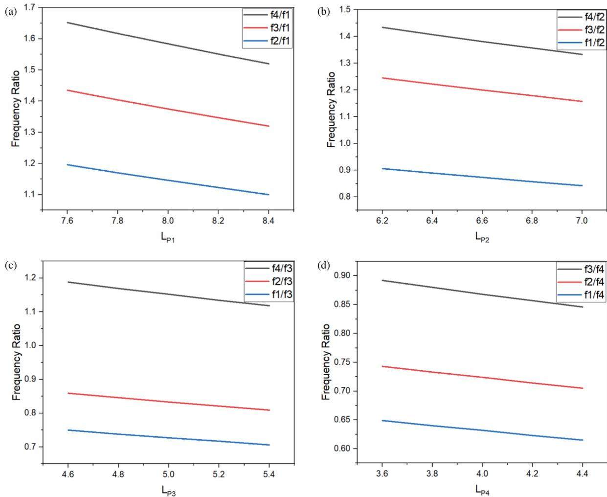
**FIGURE 7.** Design of frequency ratio using a single variable (length of the patch): (a) Frequency ratio related to  $f_1$  using  $L_{P1}$ . (b) Frequency ratio related to  $f_2$  using  $L_{P2}$ . (c) Frequency ratio related to  $f_3$  using  $L_{P3}$ . (d) Frequency ratio related to  $f_4$  using  $L_{P4}$ .
