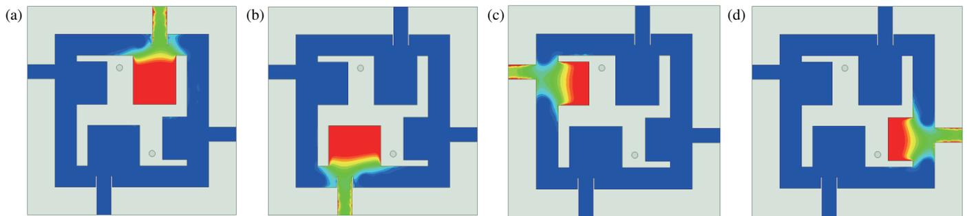
**FIGURE 5.** Electric field distribution of the proposed antenna (a) at 4.8 GHz when the input is applied at port 1, (b) at 5.5 GHz when the input is applied at port 2, (c) at 6.6 GHz when the input is applied at port 3, (d) at 7.6 GHz when the input is applied at port 4. (Note: Red colour indicates the maximum electric field intensity and blue colour indicates the minimum electric field intensity).
