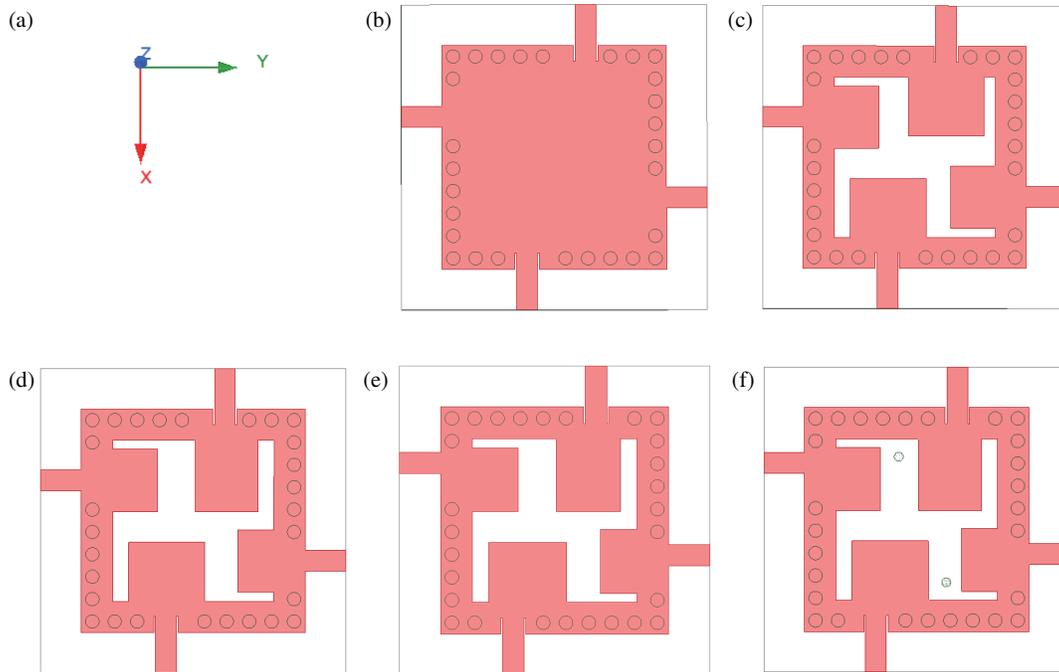
**FIGURE 1.** Design Evolution of antenna of the proposed antenna: (a) Reference directions for the antenna, (b) Stage-I: SIW Cavity, (c) Stage-II: SIW Cavity with swastik shaped slot with equal patches, (d) Stage-III: SIW Cavity with modified swastik shaped slot with center feed with unequal patches, (e) Stage-IV: SIW Cavity with modified swastik shaped slot with offset feed, (f) Stage-V-Proposed antenna: With modified swastik shaped slot with offset feed and metallic vias.
