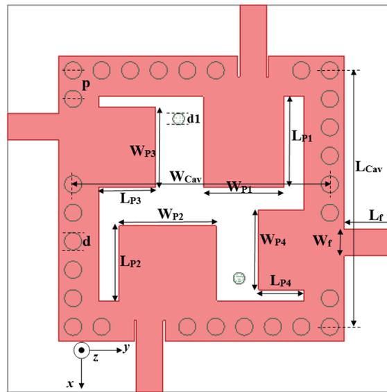
**FIGURE 3.** Structure of the antenna ( $L_{Cav} = W_{Cav} = 22.5$ ,  $p = 2.5$ ,  $d = 1.5$ ,  $d1 = 1$ ,  $L_{P1} = 8$ ,  $L_{P2} = 6.6$ ,  $L_{P3} = 5$ ,  $L_{P4} = 4$ ,  $W_{P1} = W_{P3} = W_{P4} = 7$ ,  $W_{P2} = 8.5$ ,  $L_f = 4.5$ ,  $W_f = 2.33$ ,  $hs = 0.787$ ) (all dimensions are in millimeters).
