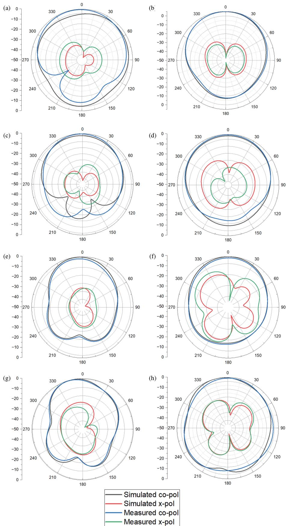
**FIGURE 10.** Simulated and measured normalized radiation patterns at resonant frequencies of: (a) 4.8 GHz ( $\Phi = 0^\circ$ ), (b) 4.8 GHz ( $\Phi = 90^\circ$ ), (c) 5.5 GHz ( $\Phi = 0^\circ$ ), (d) 5.5 GHz ( $\Phi = 90^\circ$ ), (e) 6.6 GHz ( $\Phi = 0^\circ$ ), (f) 6.6 GHz ( $\Phi = 90^\circ$ ), (g) 7.6 GHz ( $\Phi = 0^\circ$ ), (h) 7.6 GHz ( $\Phi = 90^\circ$ ).
