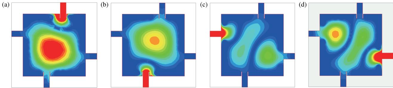
**FIGURE 2.**  $E$ -field distributions of the unperturbed cavity resonator. (a)  $TE_{110}$  mode at 6.83 GHz with input at port 1, (b)  $TE_{110}$  mode at 6.83 GHz with input at port 2, (c)  $TE_{120}$  mode at 11 GHz with input at port 3, (d)  $TE_{120}$  mode at 11 GHz with input at port 4.
