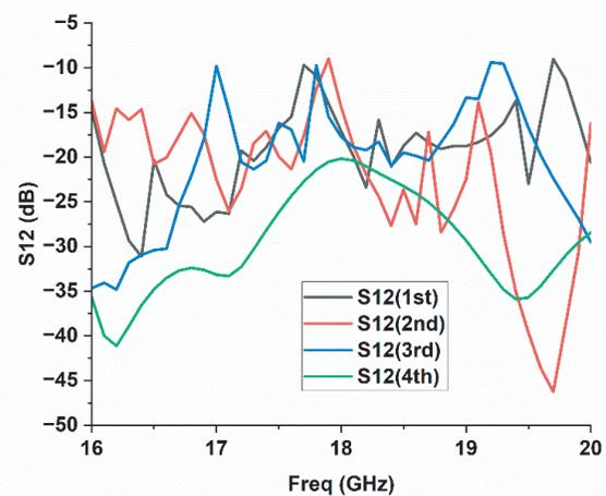
**FIGURE 3.** Comparison of  $S_{12}$  of 4 stages of development of MIMO antenna.
