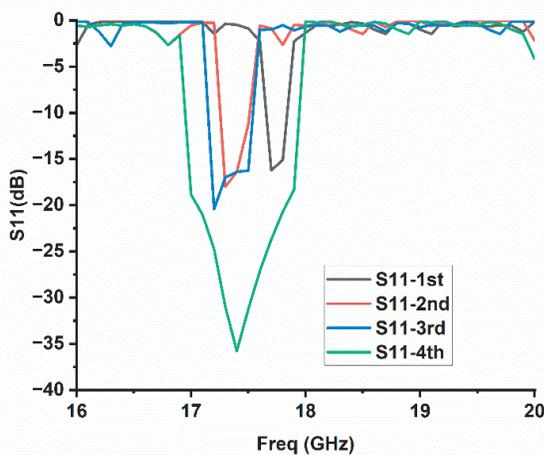
**FIGURE 2.** Comparison of  $S_{11}$  of 4 stages of development of MIMO antenna.
