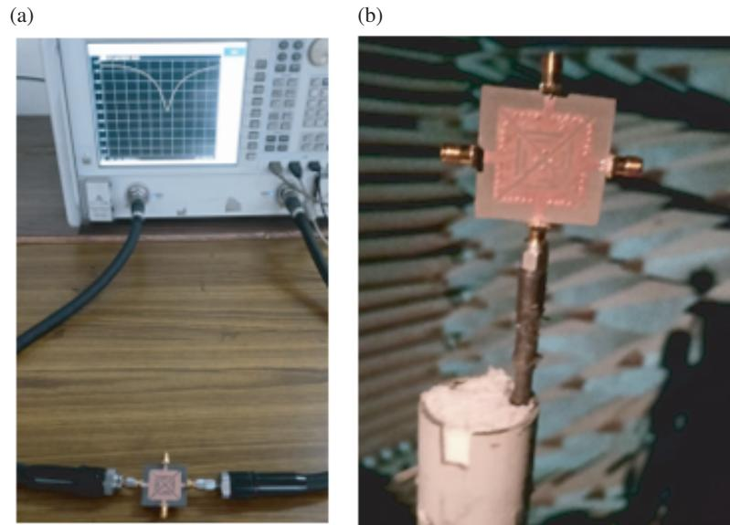
FIGURE 13. Fabricated antenna under testing. (a) VNA. (b) Anechoic chamber.
