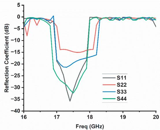
FIGURE 6. Reflection Coefficient of MIMO antenna (simulated).
