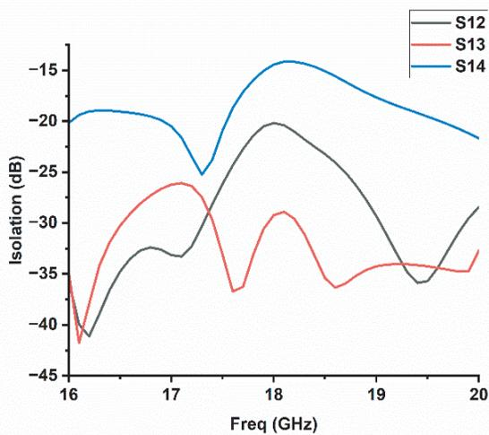
FIGURE 5. Isolation of MIMO antenna (simulated).
