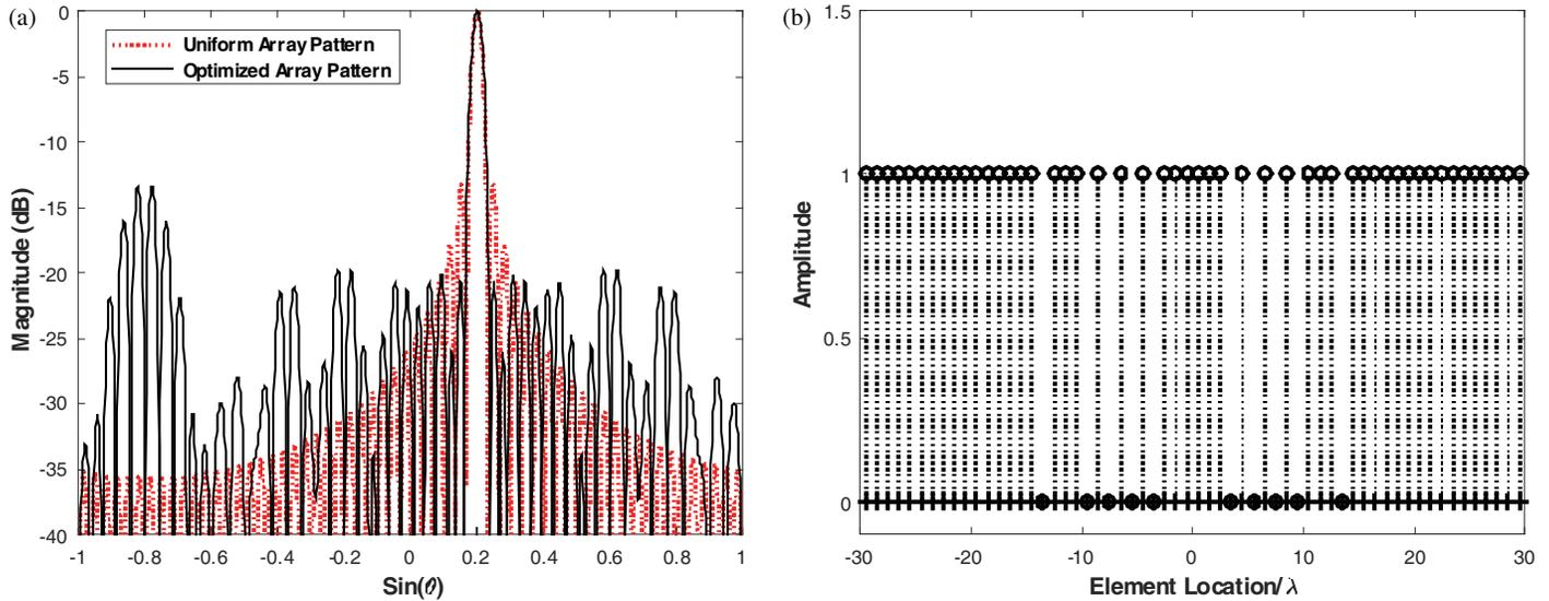
FIGURE 4. (a) Radiation patterns of both uniform and proposed arrays. (b) Optimized binary.
