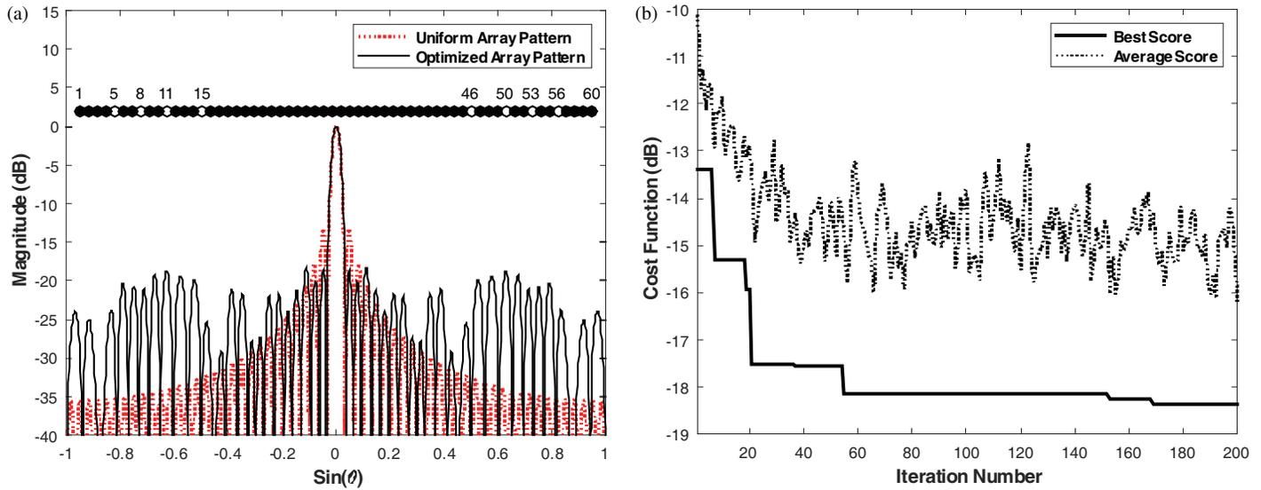
FIGURE 2. (a) Radiation pattern of the existing thinned array and (b) The cost function for 60 array elements and un-scanned main beam  $u_o = 0^\circ$ .
