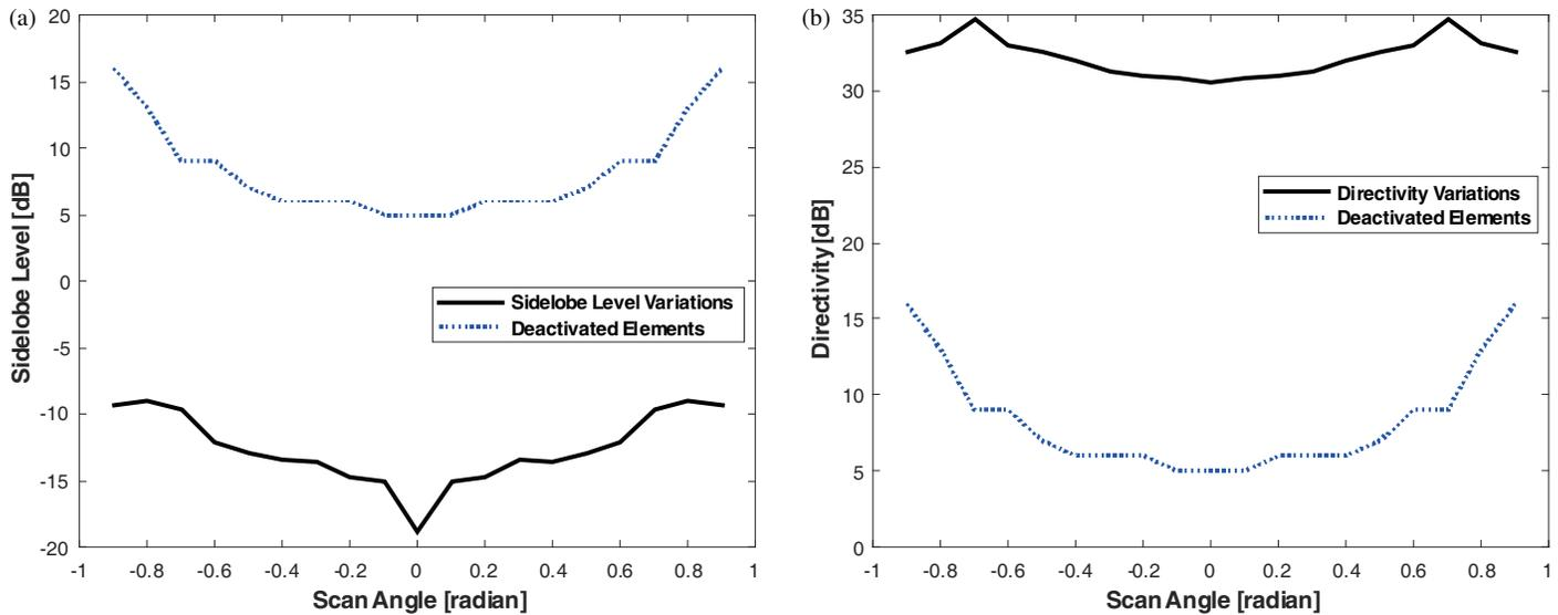
FIGURE 6. Variations of the sidelobe level and directivity versus the scanned angle.
