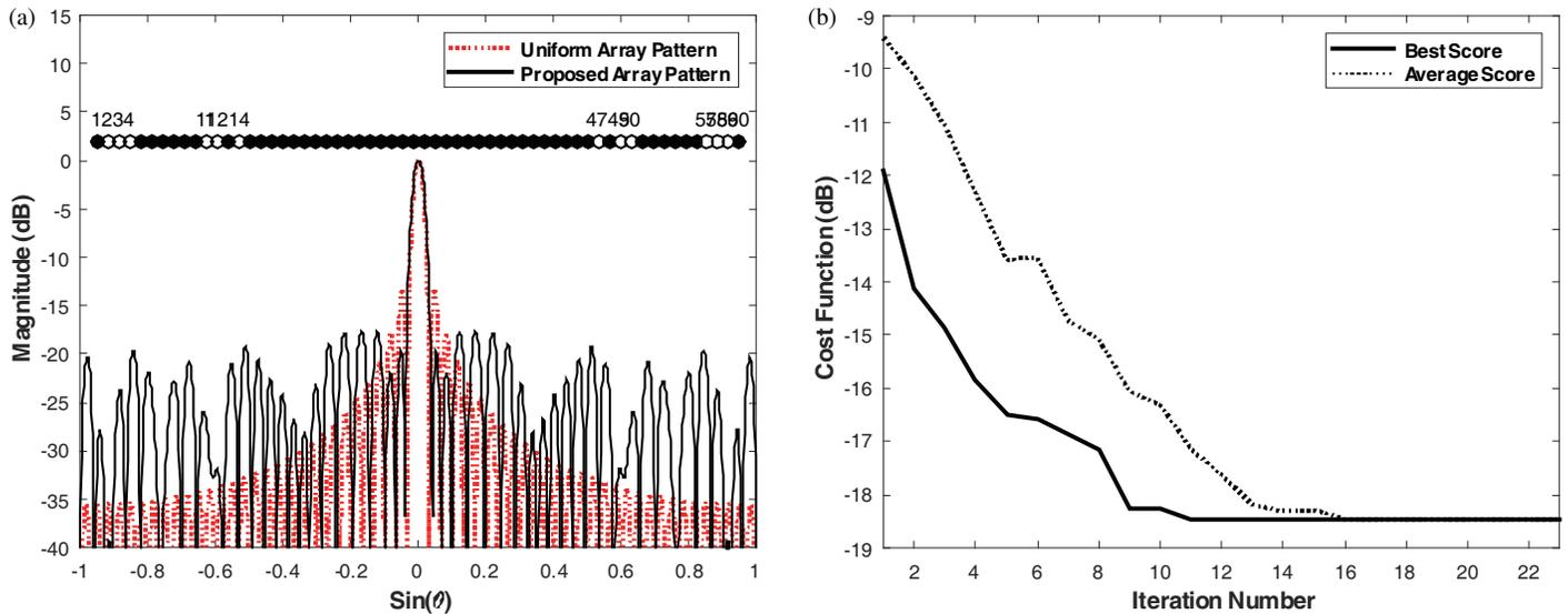
FIGURE 3. (a) Radiation pattern of the proposed array and (b) The cost function for 60 array elements and un-scanned main beam  $u_o = 0^\circ$ .
