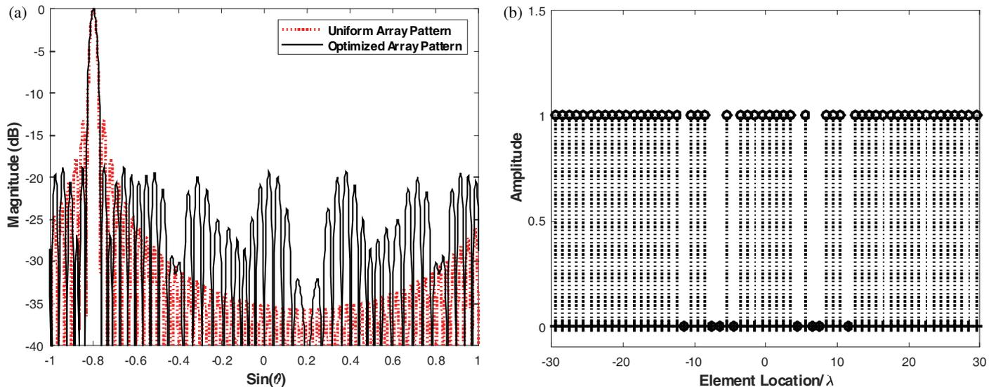
FIGURE 5. Results of the proposed array for scanned main beam  $u_o = [-0.8]^\circ$ .
