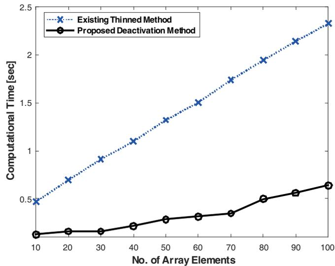
FIGURE 1. Variations of the computational time versus the number of the array elements.
