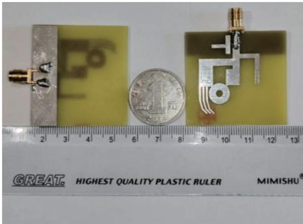
FIGURE 10. The physical model of the proposed antenna.
