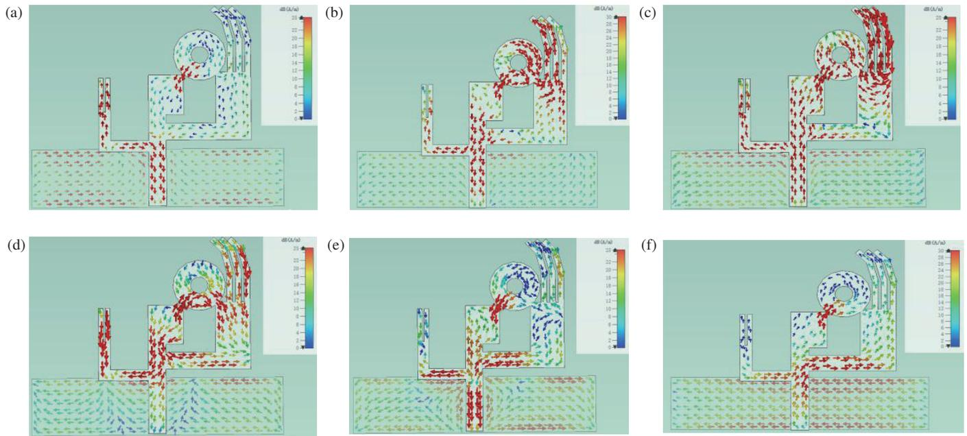
**FIGURE 6.** Mode current distribution of the improved structure: (a) mode 2 at 5.36 GHz (b) mode 3 at 3.88 GHz (c) mode 5 at 3.32 GHz (d) mode 6 at 6.94 GHz (e) mode 8 at 8.46 GHz (f) mode 9 at 2.48 GHz.
