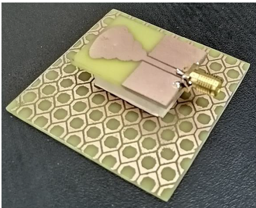
FIGURE 7. (a) Fabricated antenna. (b) Return loss simulated vs measured with reflector plate.
