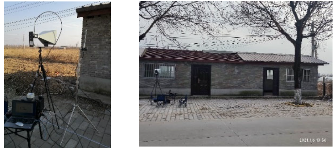
FIGURE 12. Schematic diagram of the position of the transmitting and receiving antennas during the testing process.
