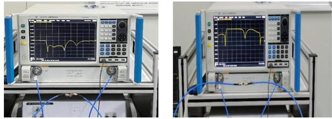
FIGURE 7.  $S$ -parameter measurement using a vector network analyzer.
