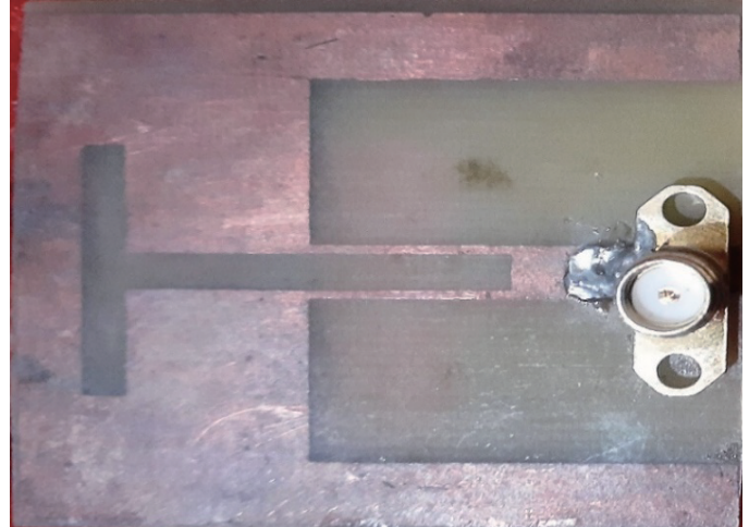
FIGURE 2. Fabricated RMPA ultra-wide band Design-1 ground plane.
