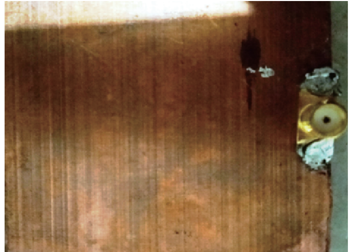
FIGURE 6. Fabricated T-shaped slotted ground plane.
