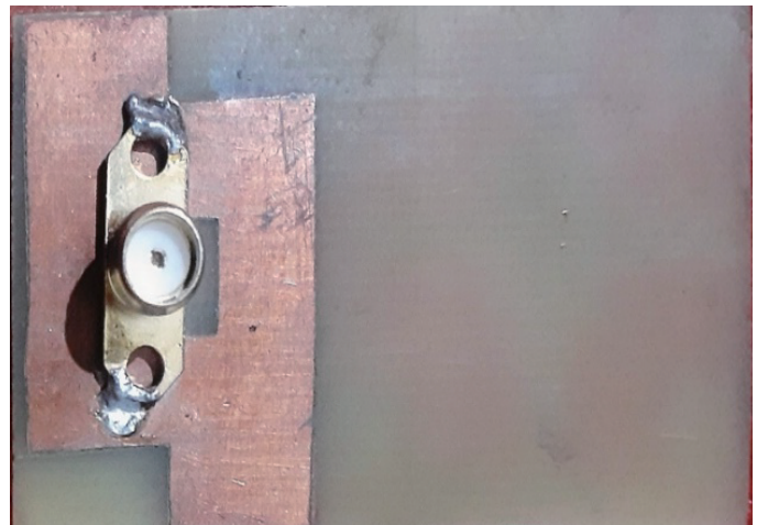
FIGURE 4. Fabricated ultra-wideband Design-2 ground plane.
