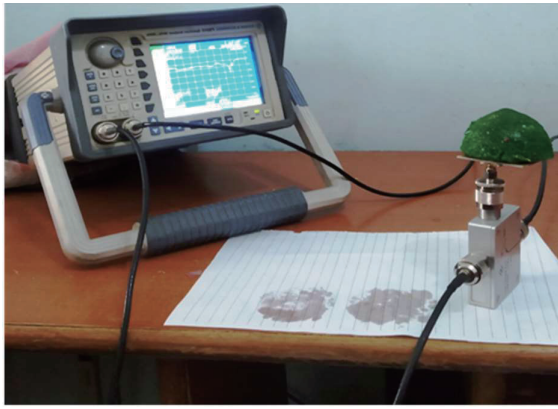
FIGURE 14. Experimental setup of brain phantom model with antenna.
