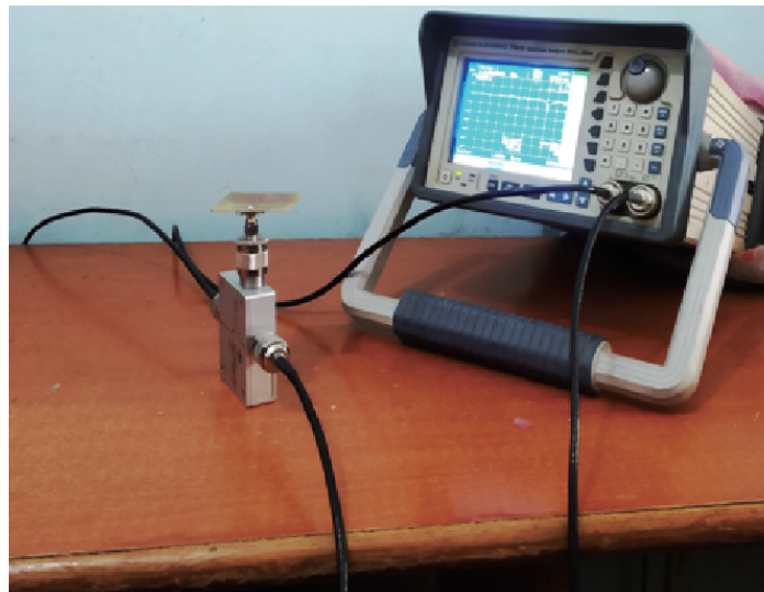
FIGURE 7. Practical setup of measurement of T-shaped slotted planner antenna.
