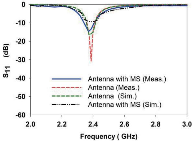
FIGURE 8. Reflection characteristics of the antenna.
