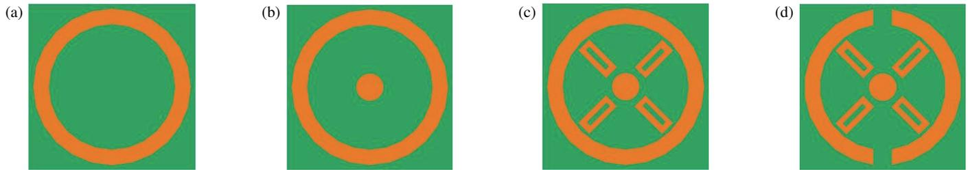
FIGURE 2. Evolution of the metamaterial unit cell. (a) CASE I. (b) CASE II. (c) CASE III. (d) CASE IV.
