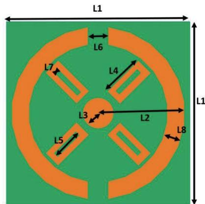
FIGURE 5. Unit cell and its dimensions ( $L1 = 23.76$  mm,  $L2 = 9.9$  mm,  $L3 = 1.98$  mm,  $L4 = 5.61$  mm,  $L5 = 3.96$  mm,  $L6 = 2.64$  mm,  $L7 = 0.66$  mm,  $L8 = 1.98$  mm).
