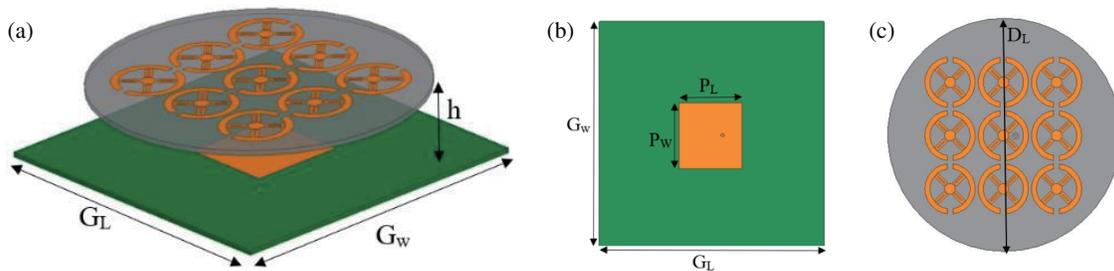
FIGURE 7. (a) 3 D Geometry of the proposed Antenna ( $G_L = 104$  mm,  $G_W = 104$  mm,  $h = 11$  mm). (b) Microstrip Patch antenna ( $P_L = 29$  mm,  $P_W = 30.5$  mm). (c) Superstrate ( $D_L = 104$  mm).
