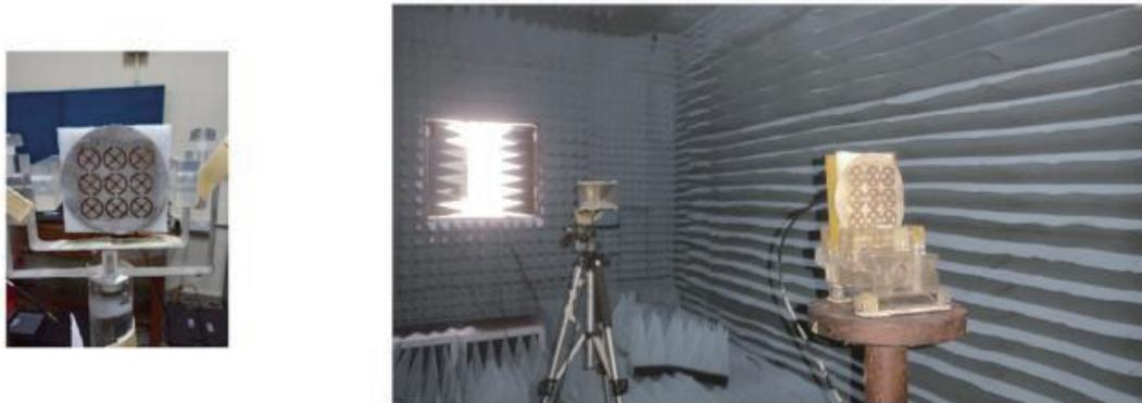
**FIGURE 13.** Fabricated prototype and the measurement setup.
