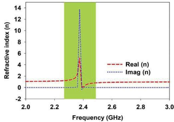
FIGURE 6. Extracted refractive index.
