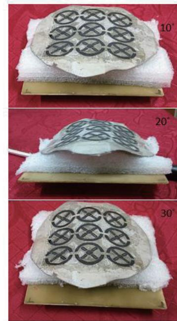
**FIGURE 15.** Practical demonstration of the superstrate at  $10^\circ$ ,  $20^\circ$  and  $30^\circ$ .
