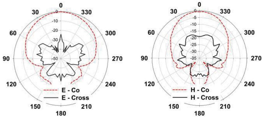
**FIGURE 12.** Measured *E*-plane *H*-plane radiation pattern.
