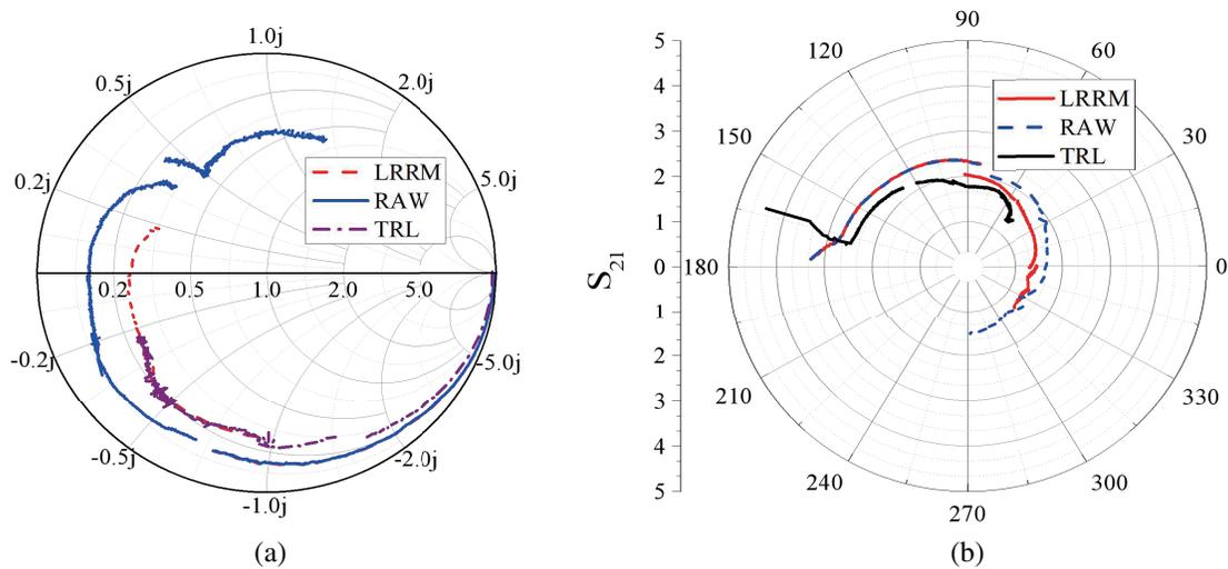
**FIGURE 14.** Comparisons of raw, LRRM and TRL ( $V_{ds} = 1\text{ V}$ ,  $V_{gs} = 0.1\text{ V}$ ) freq (0.2–66 GHz, 75–110 GHz, 110–170 GHz, 170–220 GHz). (a)  $S_{11}$ . (b)  $S_{21}$ .
