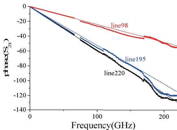
**FIGURE 12.** TRL calibration verification on “LINE” standard.
