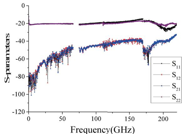
**FIGURE 13.** LRRM calibration verification on “LOAD” standard.
