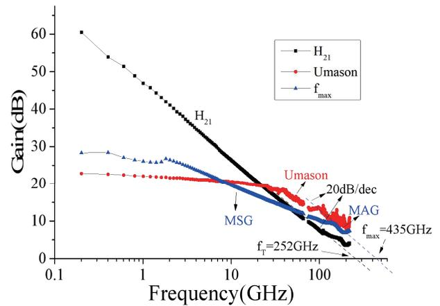
**FIGURE 16.**  $H_{21}$ , MAG/MSG and Umason versus frequency.
