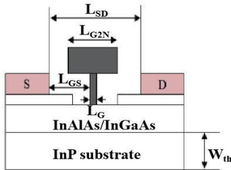
FIGURE 9. Cross section diagram of InP HEMT active area.
