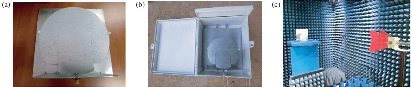
FIGURE 14. Providing the ability to measure reflection coefficient and radiation patterns: (a) the front view of the antenna prototype, (b) the antenna prototype in its housing, and (c) setting up the network analyzer and antenna prototype in the chamber room.
