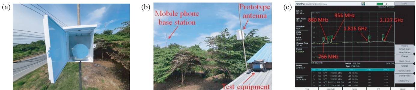
FIGURE 19. Preparing experiments for mobile signals, (a) the prototype antenna was in a plastic box, (b) a set of test equipment, and (c) the receiving signal was at a spectrum analyzer.
