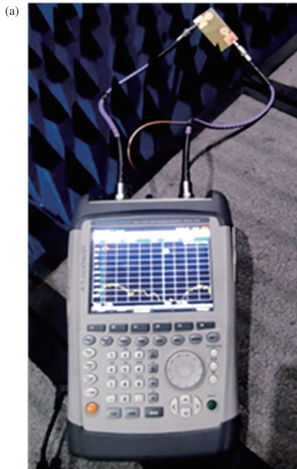
FIGURE 2. (a) Measurement setup with R&S VNA ZVH8 in the anechoic chamber. (b) Simulated and measured return loss ( S_{11} ) performance of single port and dual port triband HSRR antenna, and (c) Simulated and measured S_{12}/S_{21} , S_{22} parameters of dual port triband HSRR antenna.
