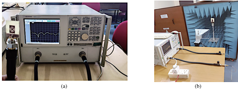
FIGURE 5. (a) Experimental set-up of proposed antenna, (a) S_{11} , (b) Gain and Efficiency.
