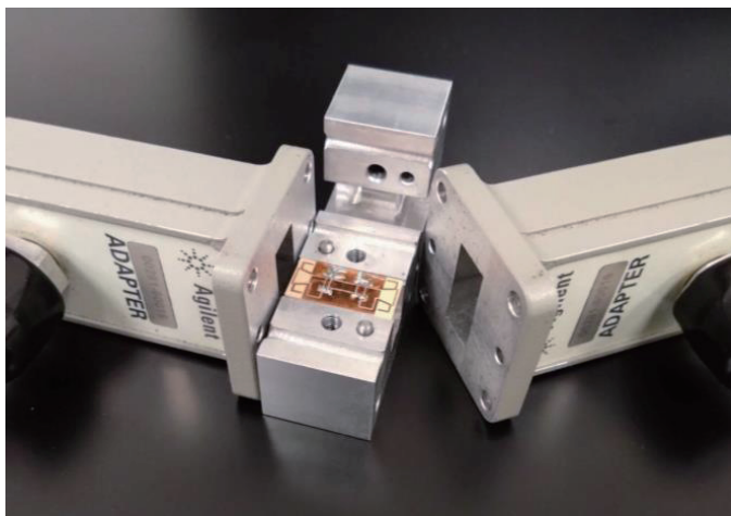
FIGURE 5. Measurement setup for the back-to-back CPW-to-RWG transition using the resonator with the impedance matching element.
