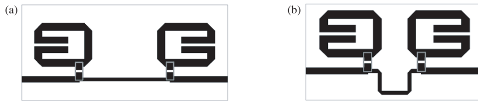
FIGURE 8. Miniaturization of the proposed equalizer: (a) The proposed equalizer; (b) The evolution process.
