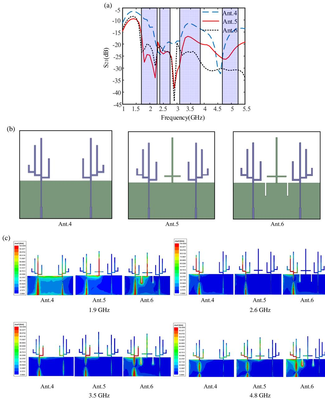
**FIGURE 3.** (a) The  $S_{21}$ -parameter curves of the quad-band MIMO antenna during decoupling stages. (b) Evolution procedures of the quad-band MIMO antenna decoupling. (c) Simulated current distributions of the quad-band MIMO antenna at 1.9, 2.6, 3.5 and 4.8 GHz during decoupling stages.
