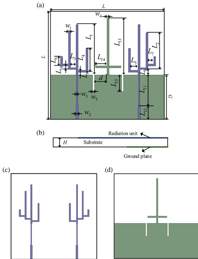
**FIGURE 1.** (a) The double-sided view. (b) Left side view. (c) Upper side view. (d) Lower side view (with  $L_1 = 27.5$ ,  $L_2 = 20$ ,  $L_3 = 3$ ,  $L_4 = 13$ ,  $L_5 = 4$ ,  $L_6 = 5$ ,  $L_7 = 3$ ,  $L_8 = 3$ ,  $L_9 = 1.5$ ,  $L_{10} = 2$ ,  $L_{11} = 17$ ,  $L_{12} = 8$ ,  $L_{13} = 31$ ,  $L_{14} = 5$ ,  $L_{15} = 9$ ,  $d = 6.5$ ,  $w_1 = 1$ ,  $w_2 = 1.2$ ,  $w_3 = 0.6$ ,  $w_4 = 1$ ,  $w_5 = 1$ ,  $L = 60$ ,  $G = 25$ ,  $H = 0.8$ , in mm).
