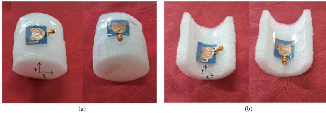
FIGURE 15. Bending of the CTWA ( x and y axis) on (a) convex surface (b) concave surface.
