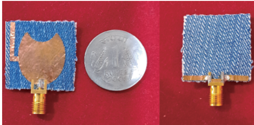
FIGURE 8. Fabricated prototype: Front and rear view of the CTWA.
