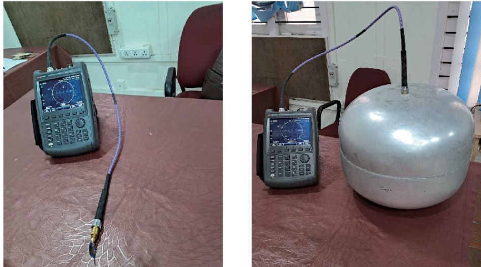
FIGURE 13. (a) Measurement set up for radiation efficiency of the proposed CTWA.
