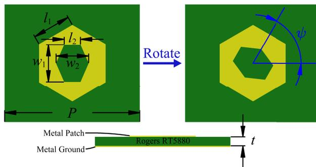
FIGURE 7. Geometry of the proposed equilateral-triangular-latticed RA element.
