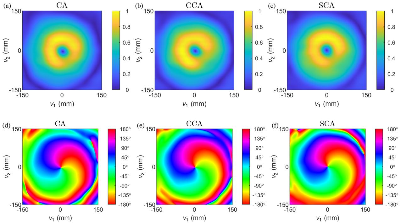
**FIGURE 9.** Simulated electric fields on the sampling plane radiated from the smooth-horn-fed equilateral-triangular-latticed CP-OAM RAs with  $\theta_F = 15^\circ$ . (a)–(c) Amplitude. (d)–(f) Phase.
