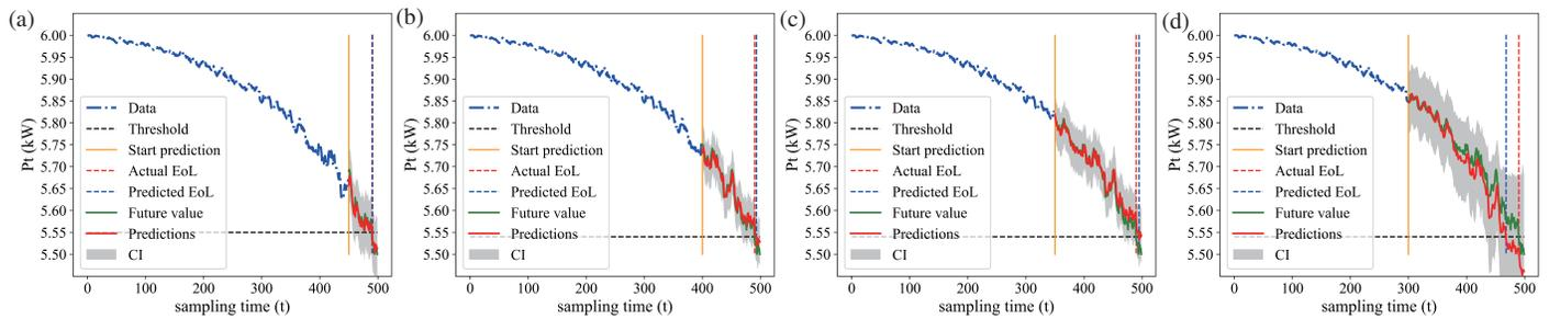
FIGURE 5. Average prediction results with 95% CI. (a)  $t_p = 450$ ; (b)  $t_p = 400$ ; (c)  $t_p = 350$ ; (d)  $t_p = 300$ .
