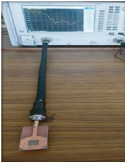
Figure 12. A fabricated antenna connected to VNA.
