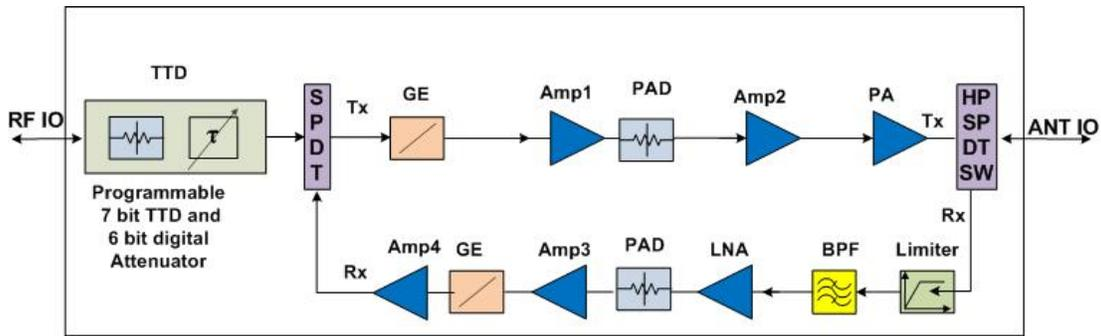
FIGURE 3. Functional block diagram of TR channel.
