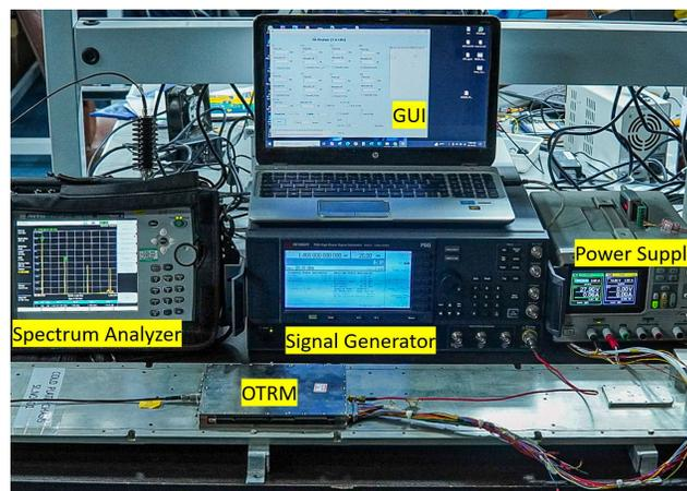
FIGURE 11. OTRM measurement setup.
