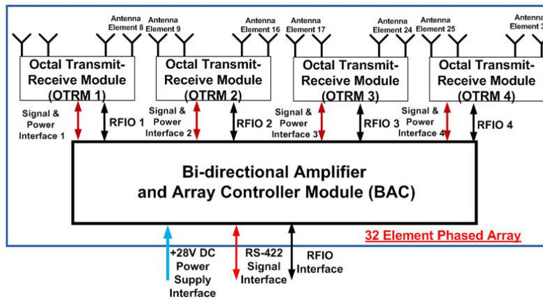
FIGURE 1. Block diagram of a 32-element phased array.
