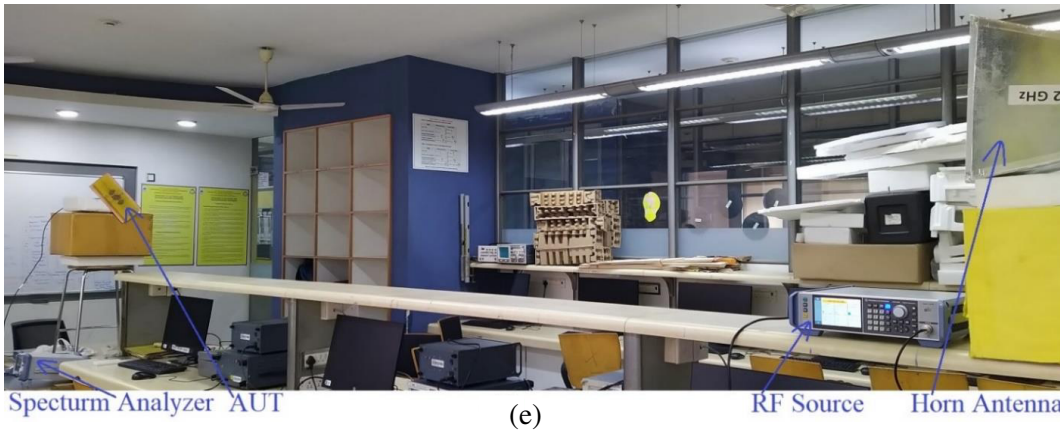
Figure 8. (a), (b) Radiation pattern, (c) field polarization plots nearer to the band start frequency of the AR BW, (d) orthogonal fields and phase plots for proximity fed gap-coupled corner truncated SMSAs along y -axis, and (e) measurement setup for the radiation pattern and broadside gain.
