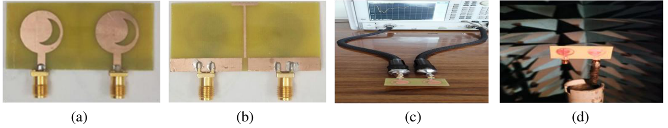
Figure 10. Fabricated antenna. (a) Front view, (b) back view, (c) vector network analyzer, (d) anechoic chamber.
